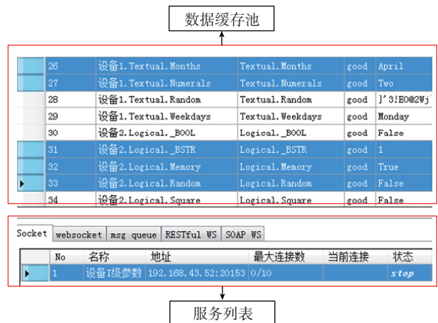
图9 实时监控系统中IMQ配置socket队列服务 Fig.9 Configuring socket queue by IMQ in real-time monitoring system
